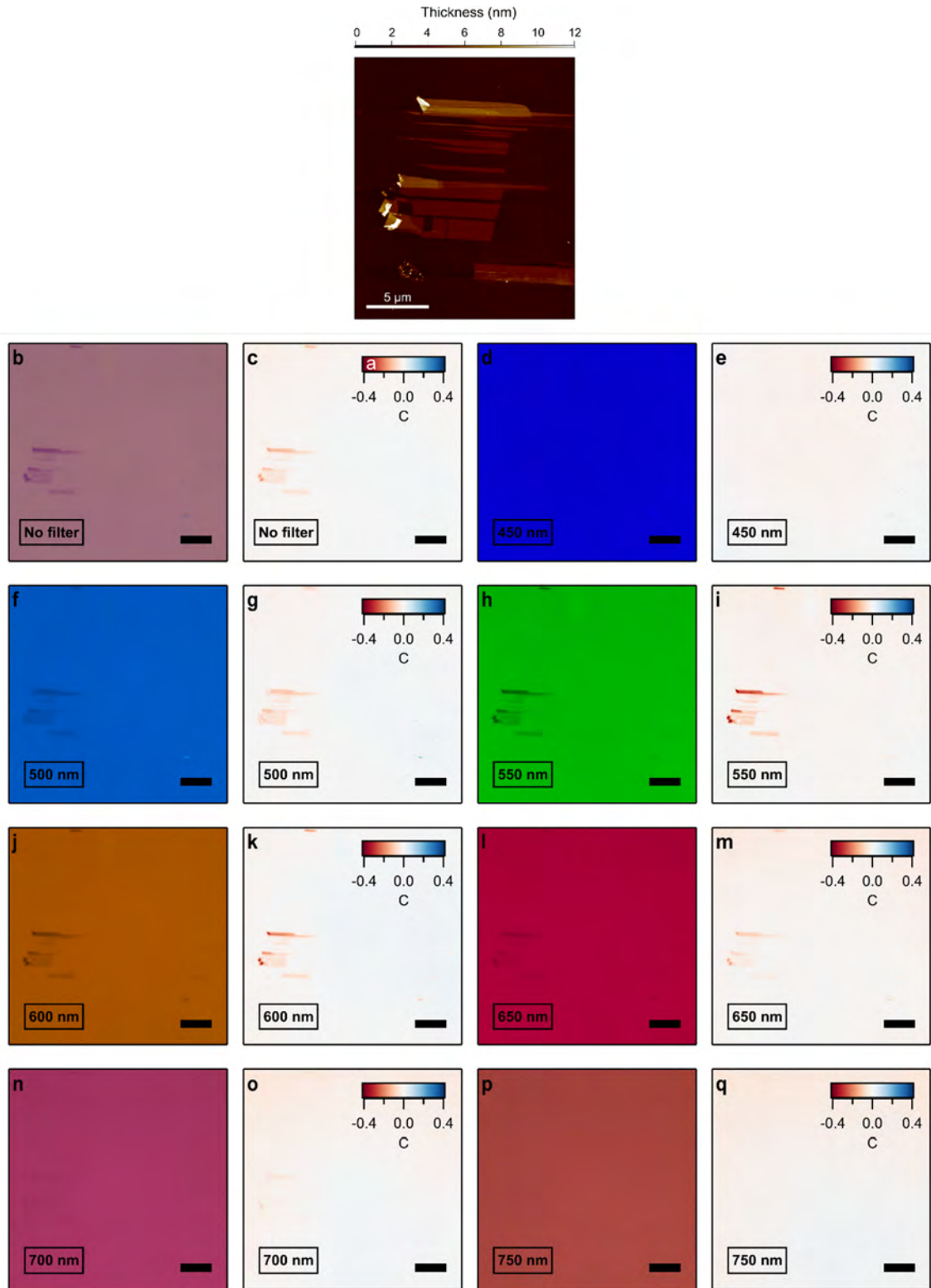
Figure S.9.- Experimental optical contrast of CrSBr thin-layers: atomic force microscopy image of the flakes (panel a), optical microscopy image without filter (panel b) and with filters (panels d, f, h, j, l, n and p). and the corresponding experimental optical contrast (panels c, e, g, i, k, m, o and q). Scale bar in contrast images: 10 \mu\text{m} .
